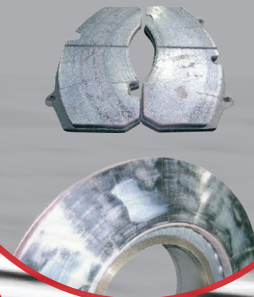
THERMAL DAMAGE & DISTORTION OF BRAKE DISC
