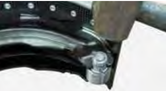
Step Two The pin is driven in and secured with two retaining rings.
