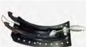
Step Three The pull-off spring is fitted.
