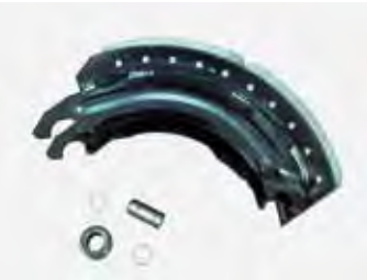
Step One The brake roller is cleaned and regreased.
