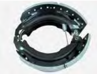
Step Four Join the two brake shoes.
